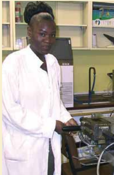
Ms Dorine Dikobe mixing plastic and wood powder in a Brabender industrial melt-mixer.
