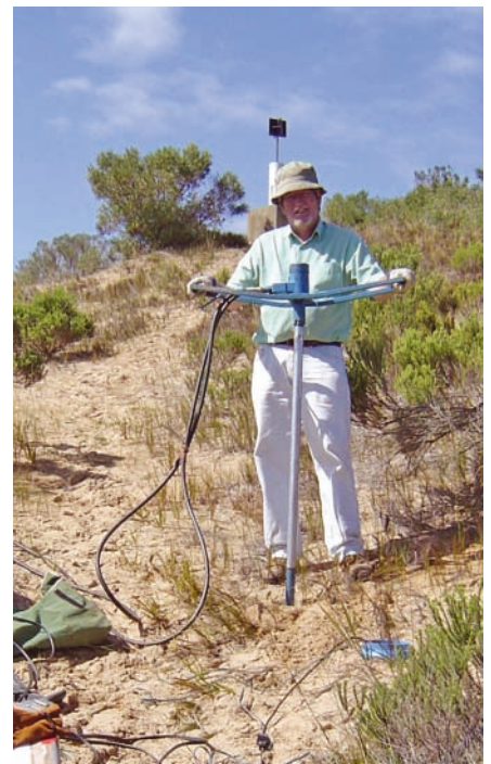
Prof. Holmes using a Dormer hydraulic corer to extract sand samples for optically stimulated luminescence dating from a dune cordon near Sedgfield.
